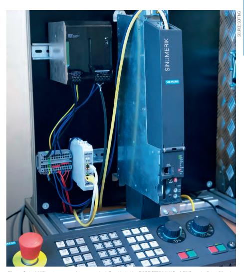
The uaGate 840D gateway can be connected directly to the SINUMERIK 840D sI CNC controller without requiring a system adaptation and any additional licenses.
