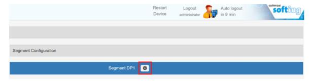
The Project Settings section contains the configured bus parameters. To take over these parameters click [Apply Configuration]. The applied configuration will become effective next time the HART IP server is activated. This means that if the HART IP server is already running you have to stop and restart the HART IP server.
