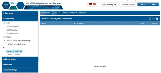
The *edgeConnector Docker* container application is available for configuration by navigating to the appropriate menu items in the *Connectivity* and *Address Spaces* sections.
