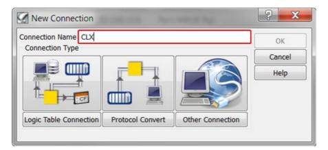
3. Click on Logic Table Connection and select the PLC/Raw and Ethernet options.
