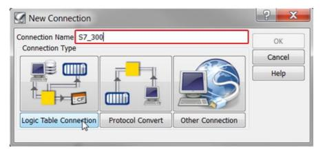
3. Click on **Logic Table Connection** and select the **PLC/Raw** and **Ethernet** options.
