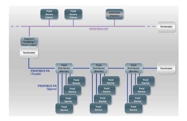
PROFIBUS PA is based on the PROFIBUS DP-V1 version. It uses the PROFIBUS DP protocol at a data transfer rate of 31.25Kbit/s and is connected to a PROFIBUS DP network using a coupling device. PROFIBUS DP then acts as a backbone network for transmitting process signals to the controller.
