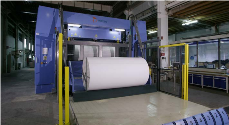
Figure 2: The paper roll slitter cuts and rewinds the produced testliners in different widths and lengths according to customer specifications
