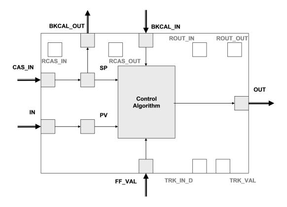
The PID takes the CAS mode if its target mode is AUTO | CAS and the upstream block is available.
