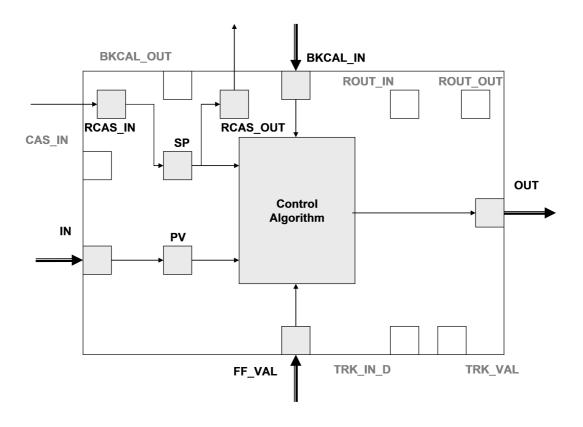
The PID takes the RCAS mode if its target mode is AUTO | RCAS and the supervisory host is available.
