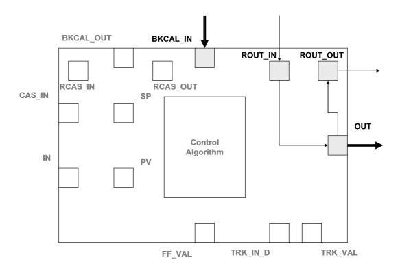
The PID takes the ROUT mode if its target mode is AUTO | ROUT and the supervisory host is available.
