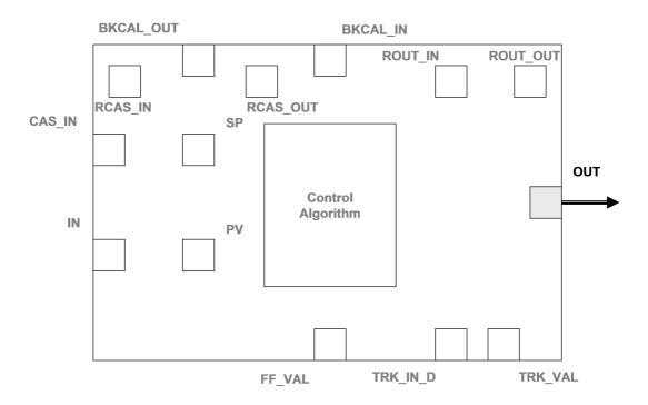
The PID takes the IMAN mode if its target mode is not OOS and the downstream block is not available.
