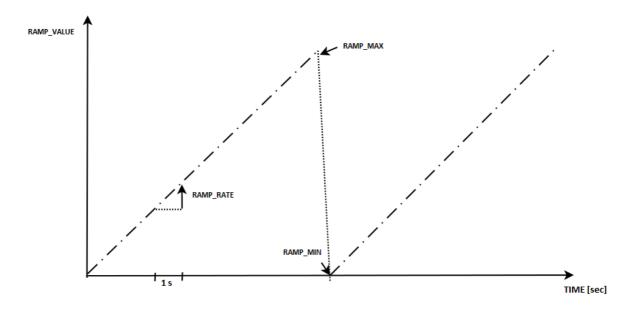
The values that impact the ramp (RAMP\_MIN, RAMP\_MAX, RAMP\_RATE) can be changed by writing to the parameters. No checks are performed any values are permitted. When a parameter is changed the ramp is not restarted. It will continue using the new value in the next transducer block execution.
