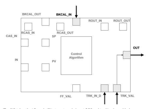
The PID takes the LO mode if its target mode is not OOS and tracking is enabled.
