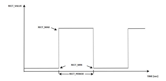
The values that impact the rectangle can be changed by writing to the parameters. No checks on parameter values are performed. The current period will continue with the old interval value and will change in the next cycle.
