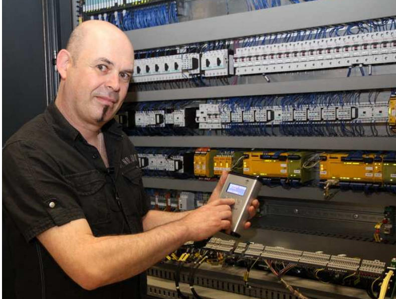
Fig. 2: The Profibus Tester 4 combines four test instruments into a single compact tool: a signal tester, a storage oscilloscope, a protocol analyzer, and a master simulator.
