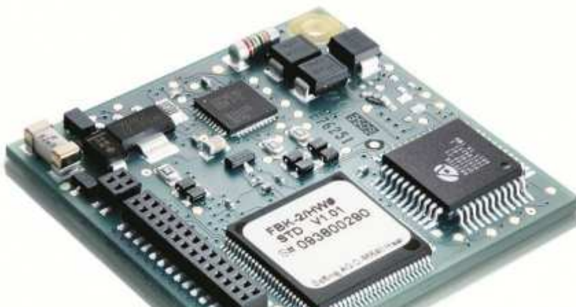
Figure 3: The Softing Fieldbus Kit product is an off-the shelf and proven solution for the rapid development of Foundation fieldbus H1 field devices.
