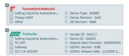
The Topology view is used to define the communication devices and the logical structure of the network.
