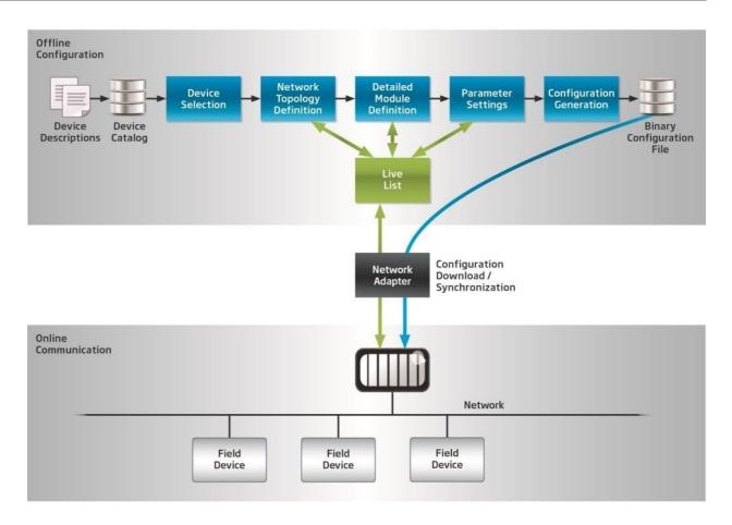
In the Communication Configuration Tool, the devices that are part of the communication application, as well as their properties can be defined. On completion of the configuration, a binary result file is created. The PROFINET controller uses the binary file to exchange data with the PROFINET devices according to the definitions made.
