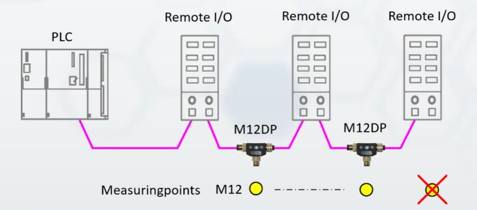
Measuring point must not be used in operation (bus termination)
