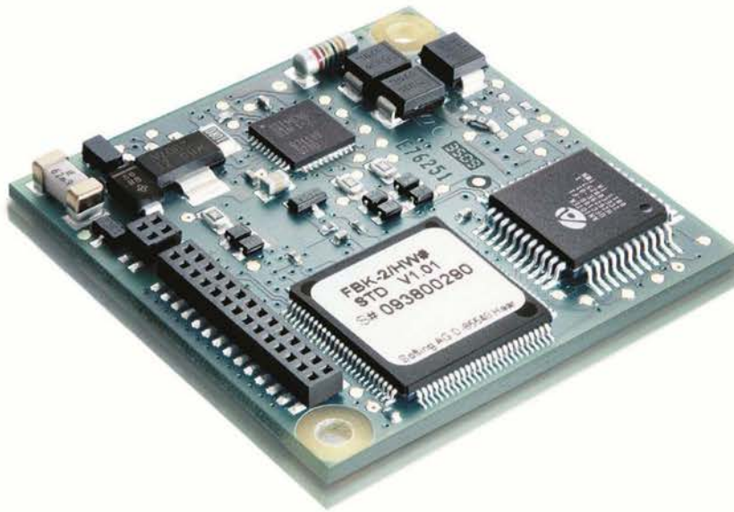
Figure 3: The Softing Fieldbus Kit product is an off-the shelf and proven solution for the rapid development of Foundation fieldbus H1 field devices.
