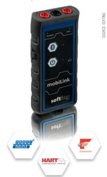
The unit provides access to three important communication protocols in process automation.
