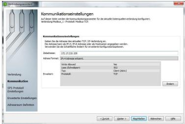
Enter the IP address of the FG-110 in the field "Target address" and click on the button "Continue".
