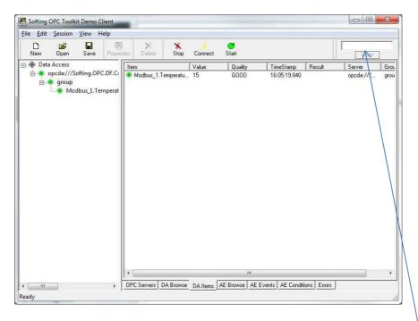
In case of a writeable Modbus register it is also possible to right a single value to the register.
