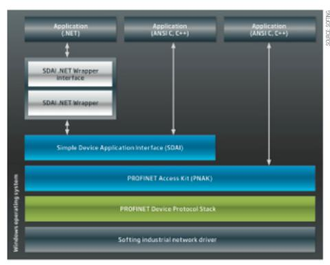
Softing's PROFINET Device Protocol Stack is ready to use in a standard Windows operating system environment.
