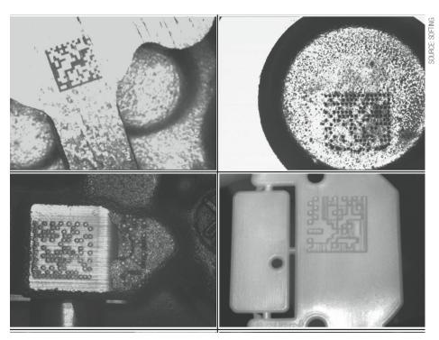
Quality differences in the markings on the components and disturbances from the environment are major challenges for the recognition performance of the Data Matrix code reader.
