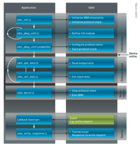
The SDAI interface allows easy implementation of the Industrial Ethernet communication. In addition to functionality for configuration, cyclic data exchange and communication termination, the SDAI also supports the handling of asynchronous events of the protocol stack, such as acyclic read and write access.
